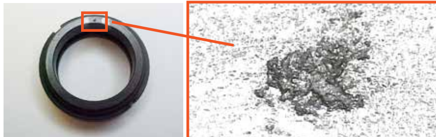
IMAGE 3: End stage of blistering, showing significant pitting and material pullout
